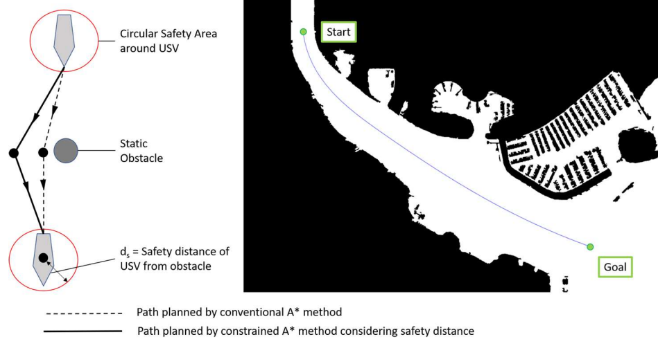
Figure 2: Schematic of the path generated from the path planner in Layer 1 (left) in (Singh et al., 2018) and the generated path along a narrow channel in the Port of Los Angeles harbor area (right).
