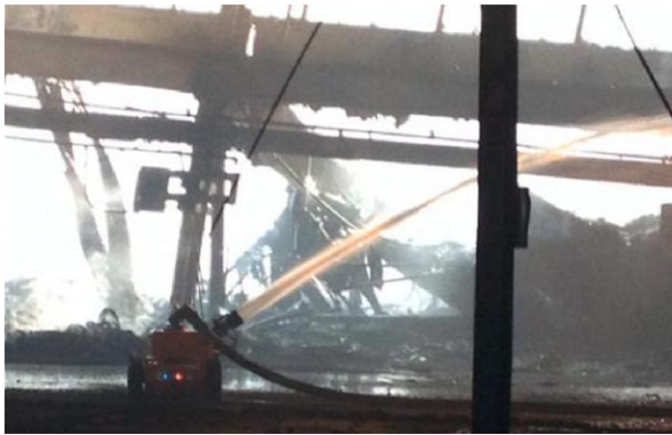
Figure 1. A firefighting robot fights a working tire fire in Illinois, USA (Min, Matson, & Khaday, 2013b).
