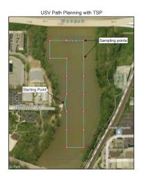
Fig. 2. USV paths planned with TSP for the Wabash River water monitoring.
